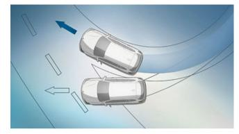
■ Dynamic Stability Control (DSC) continually assesses the vehicle's movements and optimises directional stability and traction by intervening in engine and brake management. This makes it much easier to control the vehicle, even on difficult surfaces, actively increasing driving safety.
