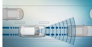
☐ **Driving Assistant** includes Forward Collision Warning which detects vehicles in front and warns the driver when if the vehicle strays from the lane of travel without indicating.
