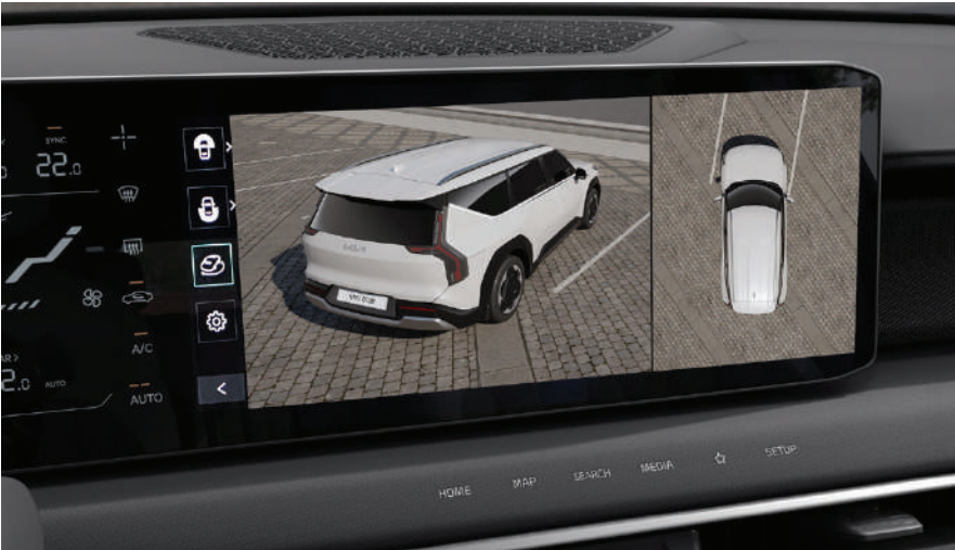
Surround View Monitor (SVM) displays a variety of views of the situation around the vehicle for safe parking.
