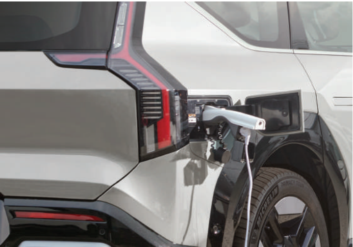
Power flows both ways in the EV9. With Vehicle-to-Load (V2L), the Integrated Charging Control Unit (ICCU) can power electric devices wherever you go. The EV9 heat pump system recaptures heat waste from the motor and other electric components to reduce winter range loss by almost 20%.
