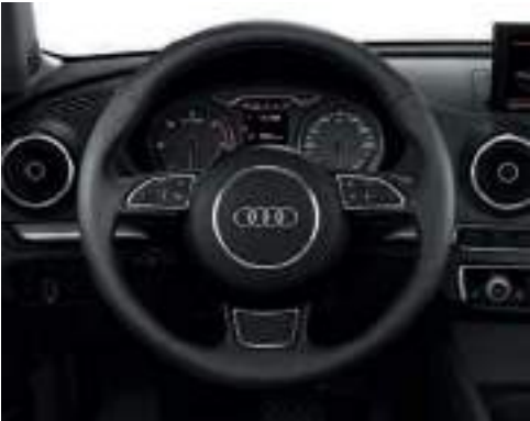
Leather-covered multifunction sport steering wheel in 3-spoke design equipment as leather-covered sport steering wheel in 3-spoke design; with multifunction buttons for operating the radio and the driver information system, phone, audio sources and navigation, optionally available with shift paddles behind the steering wheel for changing gear with S tronic
