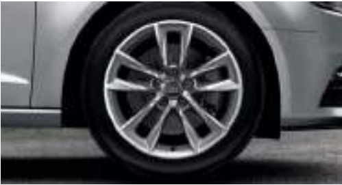
Cast aluminium wheels in 5-arm kinetic design size 7.5 J x 17 with 225/45 R 17 tyres (optionally available with run-flat tyres)
