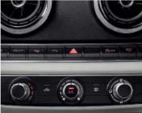
Manual air conditioning cools and heats up the vehicle passenger compartment, includes 4 air vents in the dashboard, footwell vents front and rear and defroster vents for the windscreen and side windows; features manual recirculation mode, particulate filter, continuously variable blower and manual air distribution
