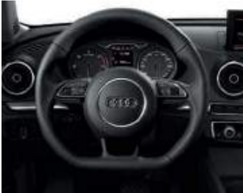
Leather-covered multifunction sport steering wheel in 3-spoke design, flattened at the bottom equipment as leather-covered sport steering wheel in 3-spoke design; with multifunction buttons for operating the radio and the driver information system, phone, audio sources and navigation, optionally available with shift paddles behind the steering wheel for changing gear with S tronic; in S3 with S3 emblem and decorative stitching in contrasting colour
