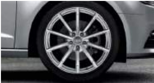
Audi exclusive cast aluminium wheels in 10-spoke design* size 7.5 J x 18 with 225/40 R 18 tyres. From quattro GmbH
