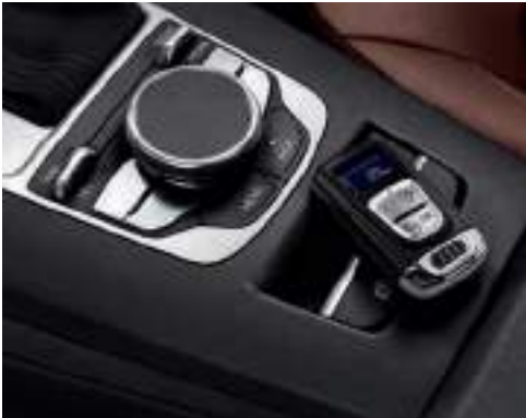
Auxiliary heating/ventilation 1 The auxiliary heating warms up the interior and removes ice from the windows; the auxiliary ventilation system supplies fresh air and lowers the temperature on the interior; with timer and departure time programming (an intelligent control function for time and energy-efficient calculation of heating duration); separate radio-operated remote control with illuminated display
