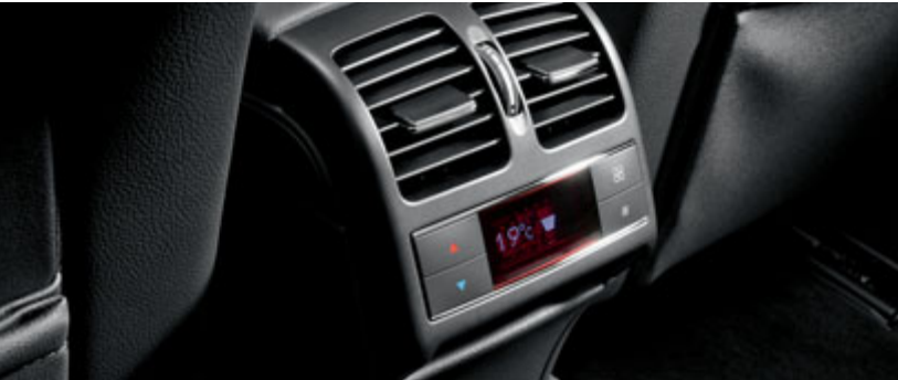
Bedieningspaneel automatische 3-zone comfortairconditioning THERMOTRONIC achter.
