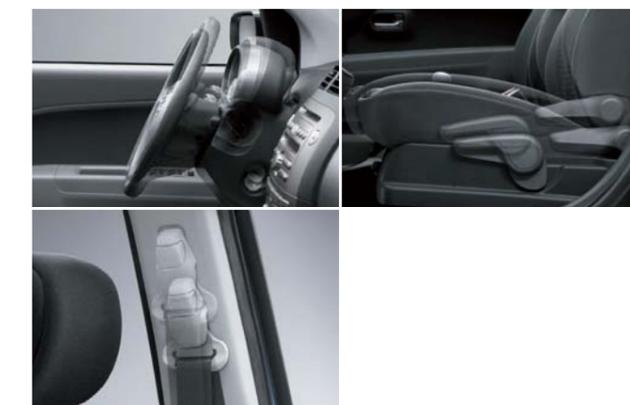
A tilt-steering column, plus seat belt and seat-height adjusters, help assure you a comfortable driving position.
