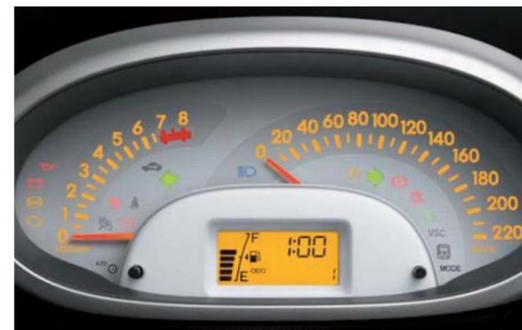
Distinctive double meters are positioned on the steering column close to the driver for visibility suited to driver physique. Illustrated meters are for 1.3-litre engine models.
