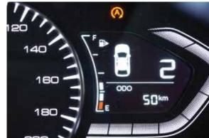
The Intelligent shift reminder in manual transmission indicates the optimum time to shift gears up or down providing greater fuel economy.
