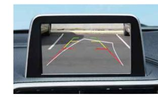
The dynamic reverse guidelines trace the vehicle's trajectory and assist in steering conveniently without colliiding into obstacles.
