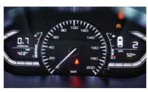
The digital RPM screen provides you with all the vehicle information without letting go of the steering wheel. It indicates fuel consumption pattern, distance to empty, trip meter, gear shift reminder for manual drive and all door open indicator to ensure safety and ease of mind.
