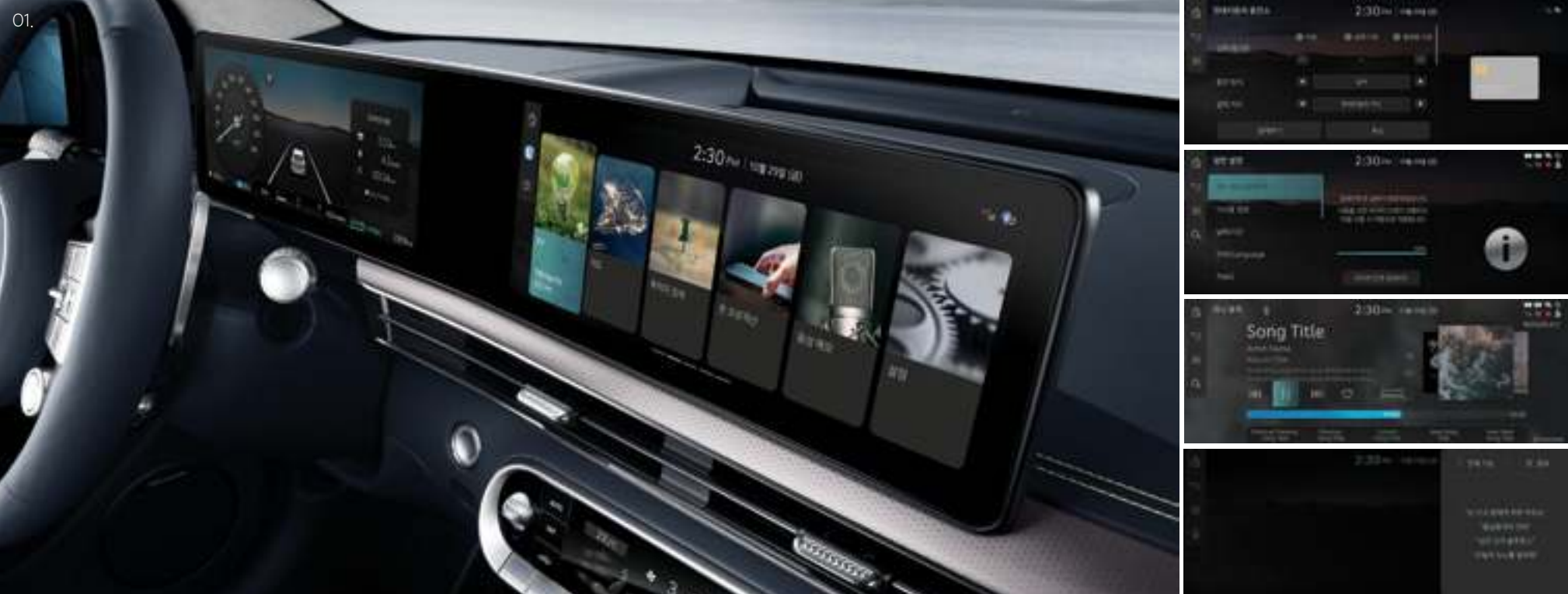
01. 12.3” Infotainment System _ The next generation connected car Integrated Cockpit (ccIC) infotainment system provides the driver with a high-tech and modern mobility experience through a panoramic display that intuitively links the digital instrument cluster, navigation system, and head-up display contents seamlessly.
