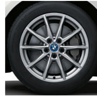
■ 17" light alloy wheels V-spoke style 851 Silver Grey uni, wheel size 7.5J x 17 with 225/55 R17 tyres. 1
